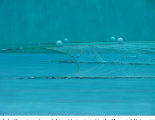
Lake Ontario scale model trawl being tested in the Memorial University of Newfoundland flume tank, the largestin the world.
