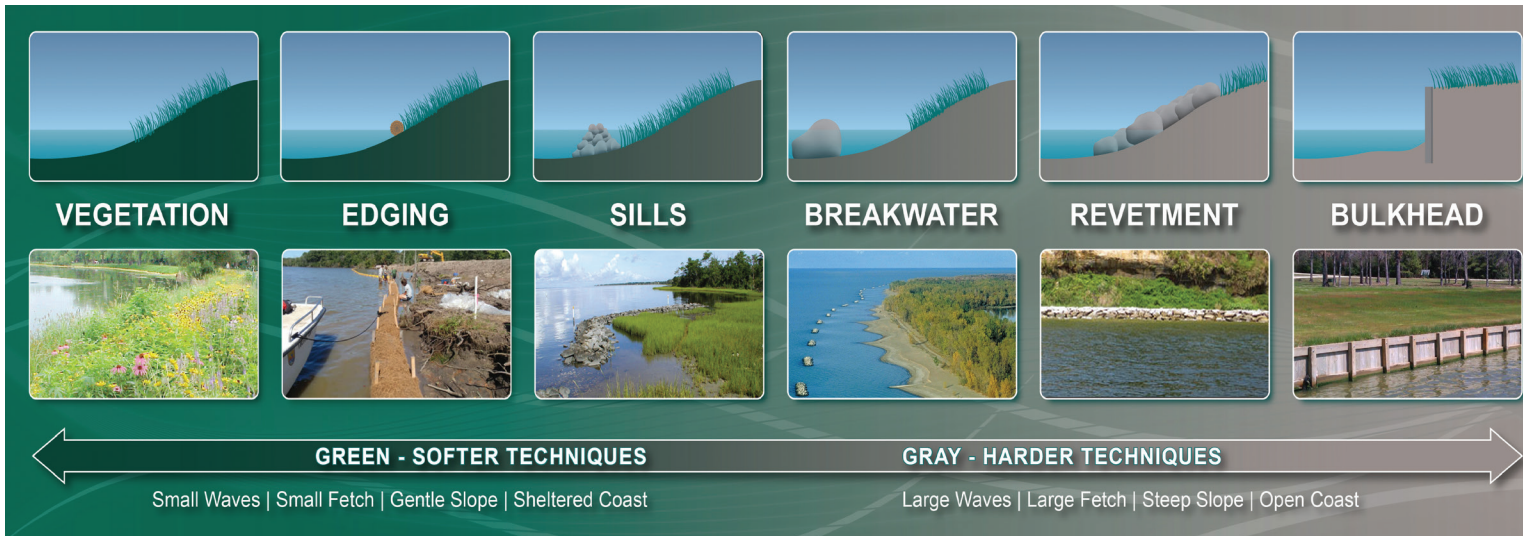
Green to gray shoreline options. Produced by Joe Ruzsala, United States Army Corps of Engineers.
